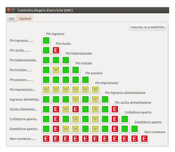
Rules can be changed by clicking on the desired square of the matrix, causing it to cycle through the choices: allowed, warning, error.
