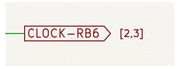
A Sheet References field with value *\${INTERSHEET\_REFS}* is automatically added to global labels, and is used to control the appearance of inter-sheet references for that label. The *\${INTERSHEET\_REFS}* text
