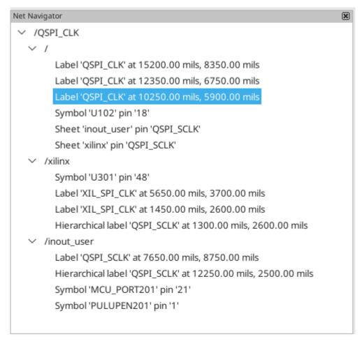
When you highlight a net in the schematic, every place where that net is shown in the schematic is listed in the net navigator panel. All labels, symbol pins, and sheet pins connected to the net are listed. Each occurrence is sorted under its schematic sheet. Clicking on an occurrence displays that item in the editing canvas. Show or hide the net navigator with **View**  $\rightarrow$  **Show Net Navigator**.
