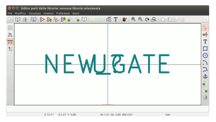
The blue cross in the center is the symbol anchor, which specifies the symbol origin i.e. the coordinates (0, 0). The anchor can be repositioned by selecting the 400 button and clicking on the new desired anchor position.
