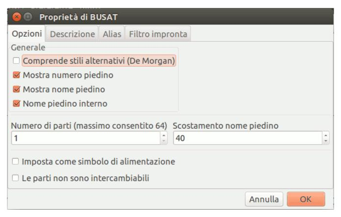
It is important to set the **number of units** and check **all units are interchangeable** and **has alternate body style**, as applicable, because these settings affect how pins and graphics are added to each symbol unit.
