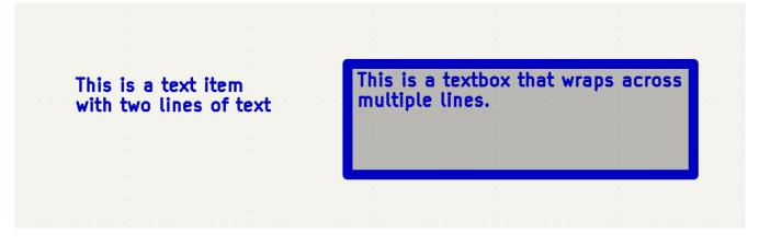
Both kinds of text item support multiline text and basic formatting features, but text boxes wrap text to fit in the outline and have additional formatting options. All text has adjustable fonts, color, size, bold and italic emphasis, left and right alignment, and vertical and horizontal orientation. Text boxes additionally support horizontal centering, vertical alignment options, and colored borders and fill.
